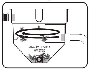
allowing the water to enter at a tangent into the first chamber or "vortex". This creates a spinning motion that forces larger, denser solids to the sides of the filter which allows them to settle at the bottom of the filter. Even troublesome solids, such as leaves, can be removed easily in this manner.
