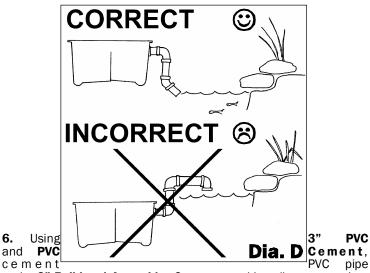
to the 3" Bulkhead Assembly. Construct and install an appropriate run of pipe to return water to your pond or waterfall. (We recommend the use of hard PVC ONLY to prevent collapse of line.) (Diagram D)
