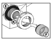
Unscrew the nut from the 2" Bulkhead (E). Place the bulkhead into the Waste Drain (K) with the gasket on the inside of the tank. While holding the bulkhead in place, thread the nut over the exposed threads until snug. Thread the 2" Male Adapter (F) into the 2" Bulkhead (E). Handtighten only.
