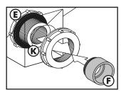
Unscrew the nut from the  $1\frac{1}{2}''$ Bulkhead (E). Place the bulkhead into the Waste Drain (K) with the gasket on the inside of the tank. While holding the bulkhead in place, thread the nut over the exposed threads until snug. Thread the  $1\frac{1}{2}''$  Male Adapter (F) into the  $1\frac{1}{2}''$  Bulkhead (E). Handtighten only.
