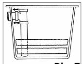
Dla. B Little Tub on a hard, level surface with the output above pond level. This is needed to allow the return water to feed back into the pond via gravity. (Diagram C)
